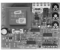
The interface board is a signal conditioner designed for the use in association a Honeywell modulation coil V7335A (Modureg). The purpose is to provide a linear conversion of a low DC voltage or current (produced by measure or control equipment) to a requested control current or voltage for the modulation coil (0-22 V-DC or 30-165 mA-DC).
