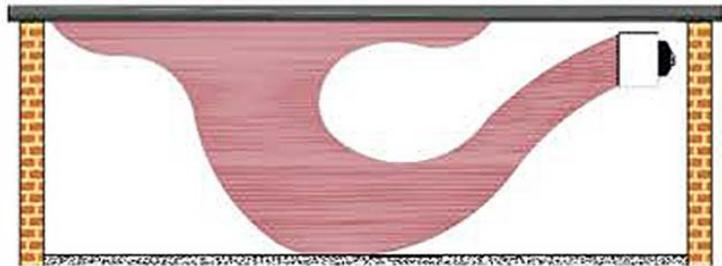
Shorter air throws reduce air distribution efficiency and require longer pre-heat times
