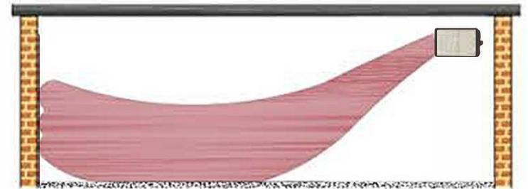
Longer air throws provide even heat distribution and reduce pre-heat times
