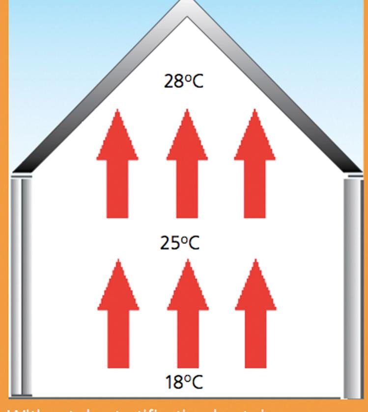
Without de-stratification heat rises resulting in poor distribution, increased heat loss and running costs.
