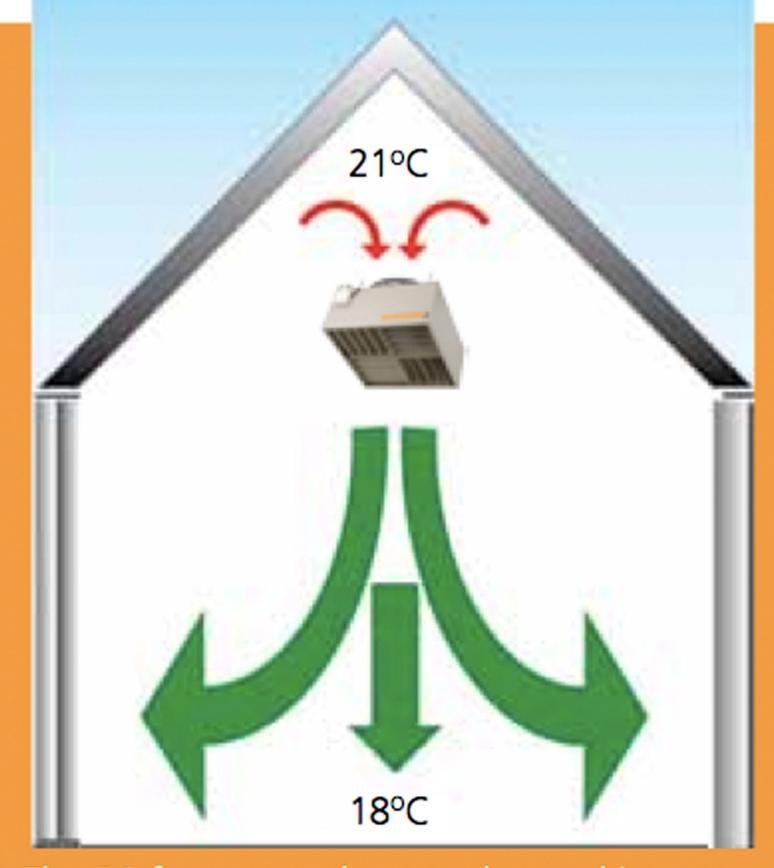
The DS fan returns heat to the working zone for improved comfort and reduced running costs.
