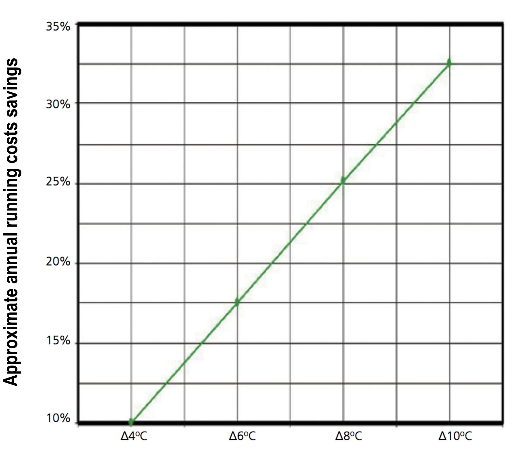
ΔT Temperature gradient from floor to roof level For effective de-stratification, sufficient fans must be installed to re-cycle heat from the full roof area.
